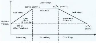
Fig 3.Stress Freezing Cycle
