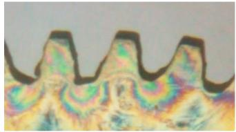
Fig 4.Fringe Pattern at the Tooth Root
