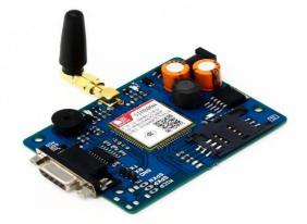
Fig -7: GSM Module
