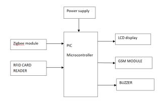
Fig -3: Block Diagram (Counter unit)
