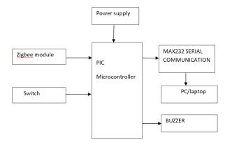
Fig -2: Block Diagram (Kitchen unit)
