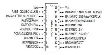
Fig -4: PIC16f690 Microcontroller
