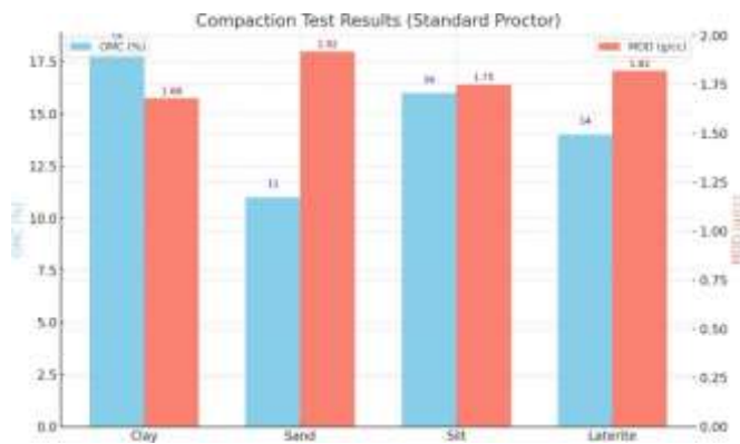
Figure 2. Compaction test results using the standard proctor method
