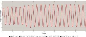
Fig -8: Source current waveform with Hybrid active power filter compensation
