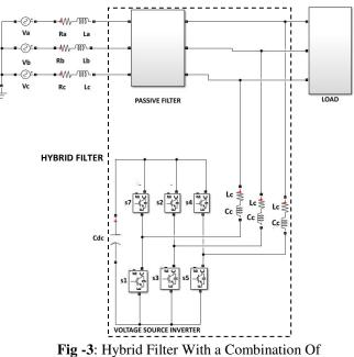
**'ig -3**: Hybrid Filter With a Combination Of Series Passive And Shunt Active Filter
