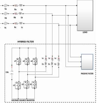
**Fig -2**: Hybrid Filter With a Combination Of Shunt Active And Shunt Passive Filter
