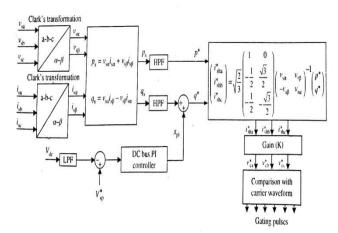
Fig -5: Modified Instantaneous Reactive Power Theory
