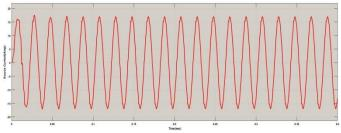
Fig -14: Source current waveform with passive filter only
