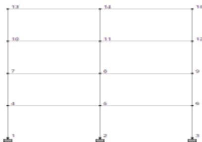
Fig. 1 2D Frame with usual columns
