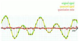
Fig the simplest way to quantize a signal is to choose the digital amplitude value closest to the original analog amplitude.
