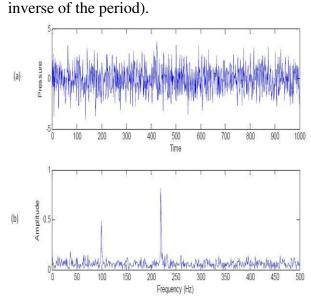
(a) The time series and (b) frequency spectrum of a signal
