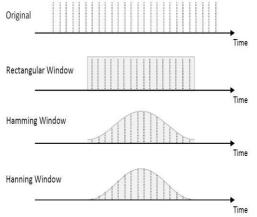
Fig The effects of different window functions on a digital signal Filtering
