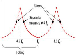
**Fig.** The black dots are aliases of each other. The solid red line is an example of adjusting amplitude vs. frequency. The dashed red
