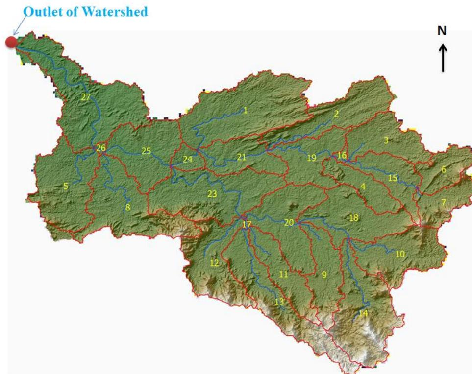
Fig – 6. QSWAT Model Delineation of 27 sub-watersheds from DEM
