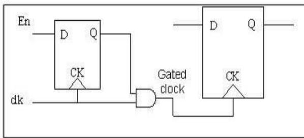
Fig1. Latch Based-clock gating
