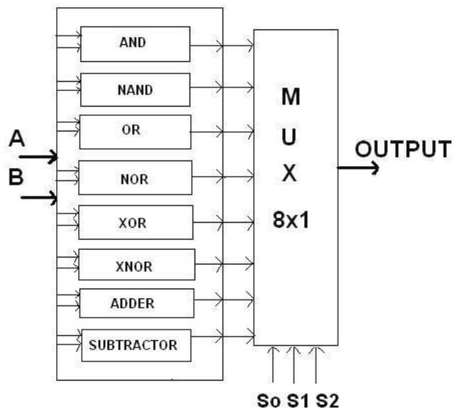
Fig3: Block diagram of ALU
