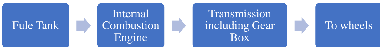
Fig 2. Flow of energy within a mechanical drive train (Prajapati et al, 2014).
