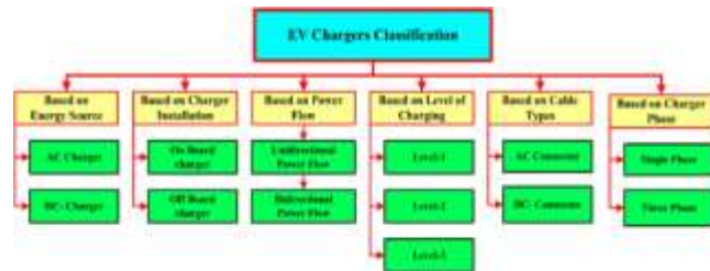
Fig. 2. Taxonomy of EV Charging Using Solar Energy with IoT-Based Data Monitoring
