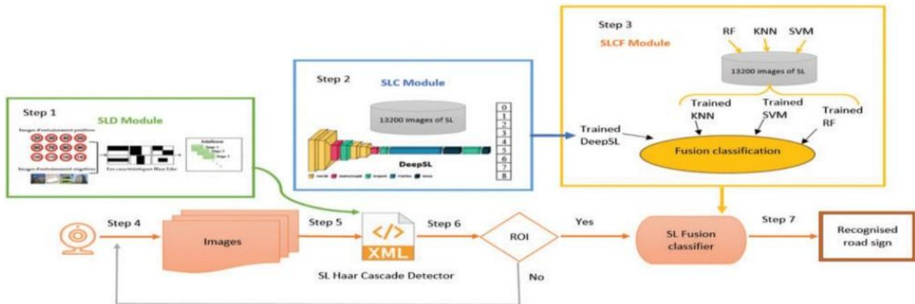
Fig. 4. Proposed speed limit recognition methodology. [3]
