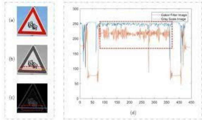
Fig. 5. (a) Traffic sign of RGB; (b) grayscale image; (c) synthetic Gabor filtered map; (d) two vector contrast graphs.
