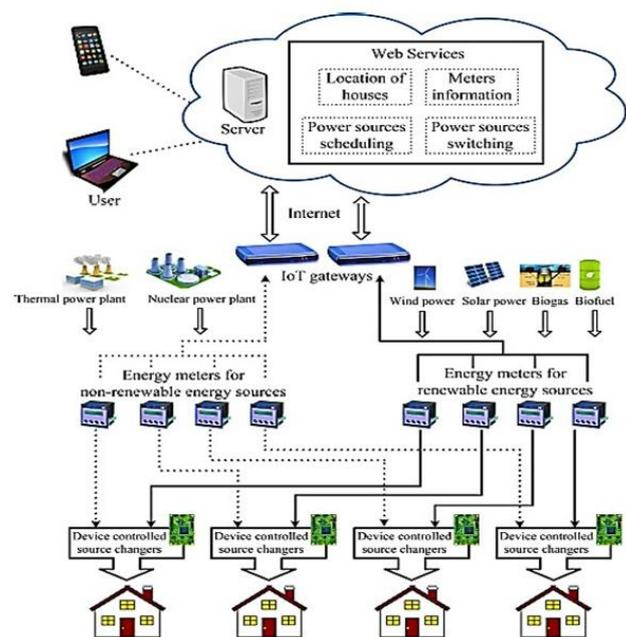
Fig 6: Web-enabled SG architecture built on top of IoT devices with web services.
