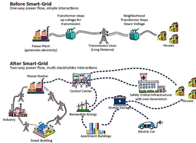
Fig. 2: Environment of the smart-grid inside the national power system
