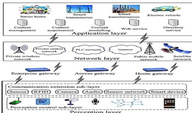
Fig 5: A perception layer, a network layer, and an application layer make up the three layers of the IOT SG system's architecture.
