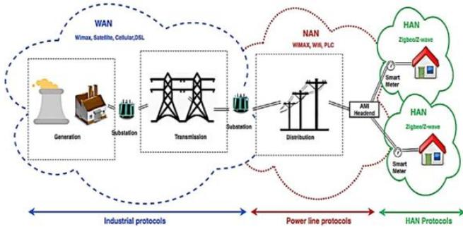
Fig 4: Illustration of the smart grid architecture
