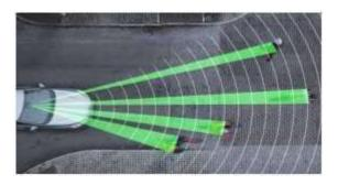
**Sensor fusion** To combine the respective outputs of RADAR and LIDAR, we use Kalman Filters. Kalman filters are unimodals and use Gaussians to represent state and uncertainty.
