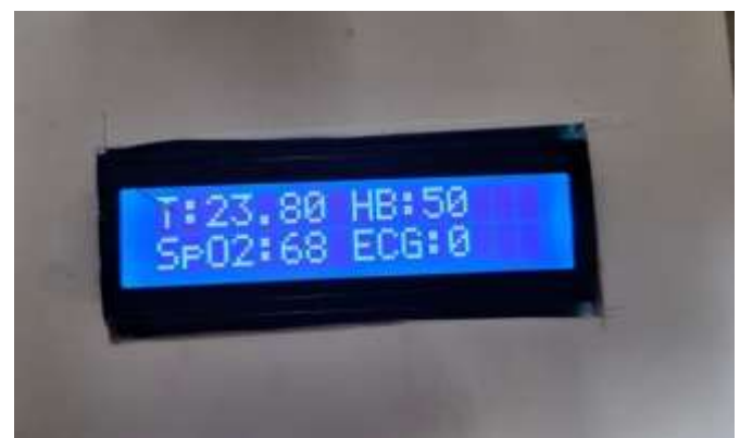
Figure 4.7: A 16X12 LCD display showing the results of temperature,heartbeat,oxygen and ECG.
