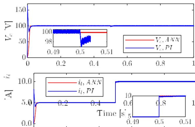
Fig. 9. Simulation results of the output voltage and current of the DC boost converter using PI and ANN-based controllers under step change of load.
