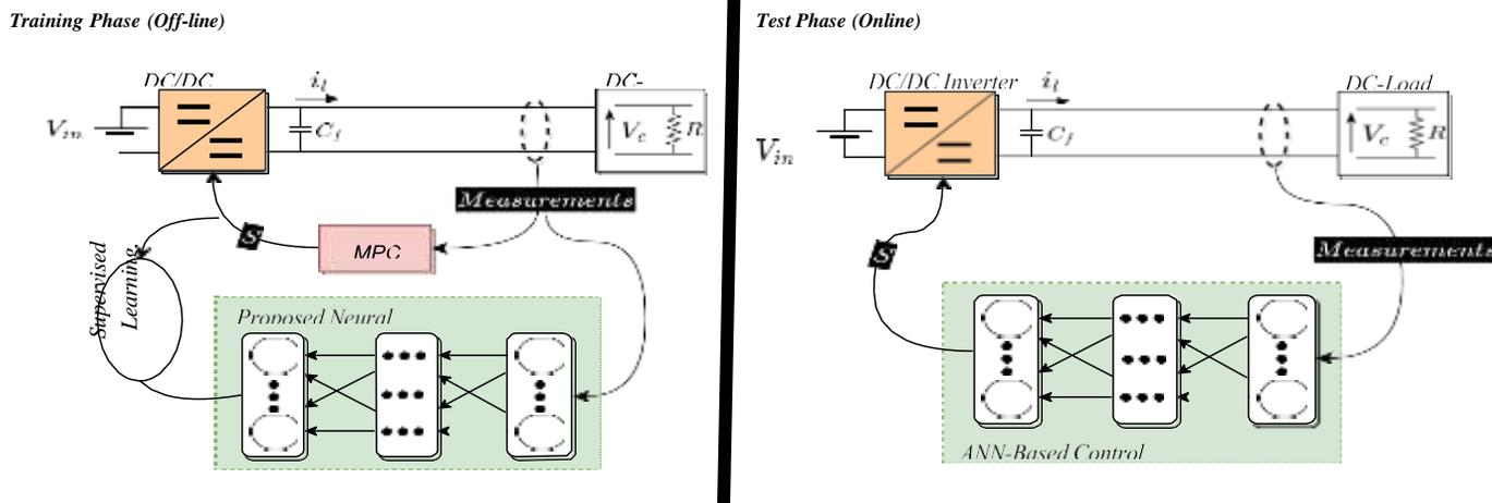
Fig. 2. Overview of the proposed control strategy. During the training phase, the classical MPC is used to control the DC/DC converter and collect the training data. In the test phase, the trained ANN is implemented to control the voltage of the converter instead of MPC [10].
