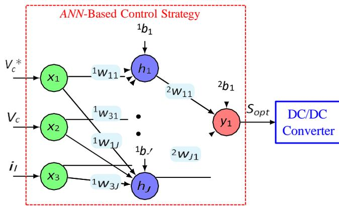
Fig. 4. Block diagram of the proposed ANN-based control scheme for the DC/DC converter. It is trained to map directly from the measured variables, namely,  $V_c^*$ ,  $V_c$ , and  $i_l$ , to the optimum switching state  $S_{opt}$ .
