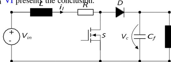
Fig. 3. Circuit diagram of the DC/DC converter.
