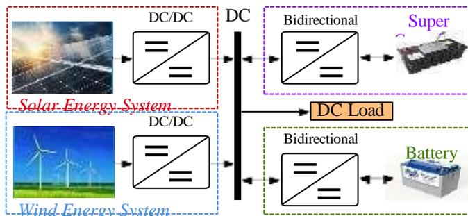
Fig. 1. Possible structure of single bus DC MG, including renewable energy sources such as solar and wind, energy storage systems, and DC load.
