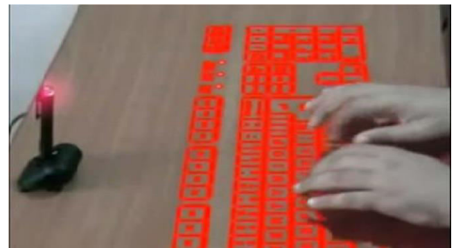
Figure 7: Diagram of Virtual keyboard Pen
