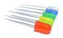
x A light-emitting diode (LED) is a semiconductor light source that emits light when current flows through it. Electrons in the semiconductor recombine with electron holes, releasing energy in the form of photons. ... Modern LEDs are availableacross the visible, ultraviolet, and infrared wavelengths, with high light output
