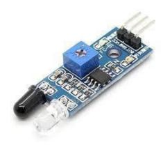
An infrared sensor is an electronic instrument that is used to sense certain characteristics of its surroundings. It does this by either emitting or detecting infrared radiation. Infrared sensors are
