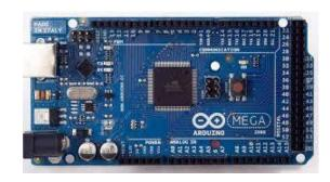
The **Arduino Mega 2560** is a microcontroller board based on the ATmega2560. It has 54 digital input/output pins (of which 15 can be used as PWM outputs), 16 analog inputs, 4 UARTs (hardware serial ports), a 16 MHz crystal oscillator, a USB connection and a power jack, an ICSP header and a reset button.
