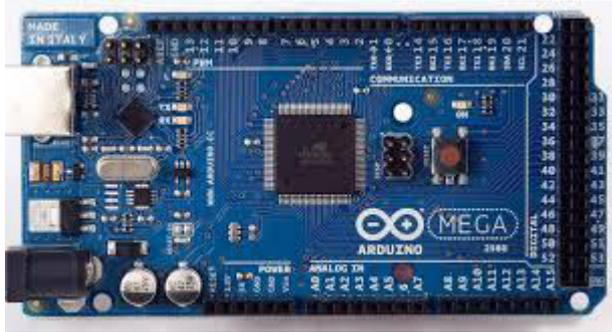
The **Arduino Mega 2560** is a microcontroller board based on the ATmega2560. It has 54 digital input/output pins (of which 15 can be used as PWM outputs), 16 analog inputs, 4 UARTs (hardware serial ports), a 16 MHz crystal oscillator, a USB connection, a power jack, an ICSP header, and a reset button.
