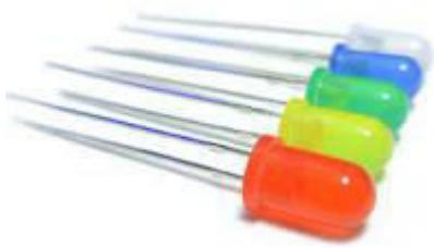
A light-emitting diode (LED) is a semiconductor light source that emits light when current flows through it. Electrons in the semiconductor recombine with electron holes, releasing energy in the form of photons. ... Modern LEDs are available across the visible, ultraviolet, and infrared wavelengths, with high light output
