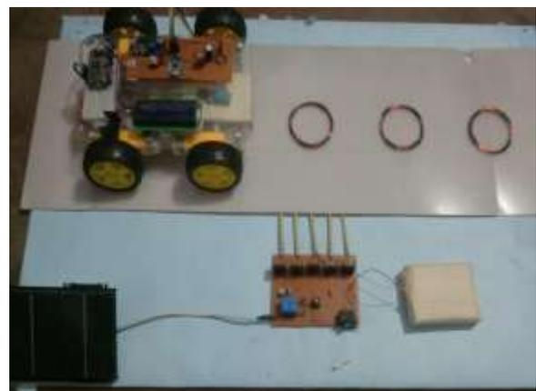
LCD Display show temperature humidity and voltage.
