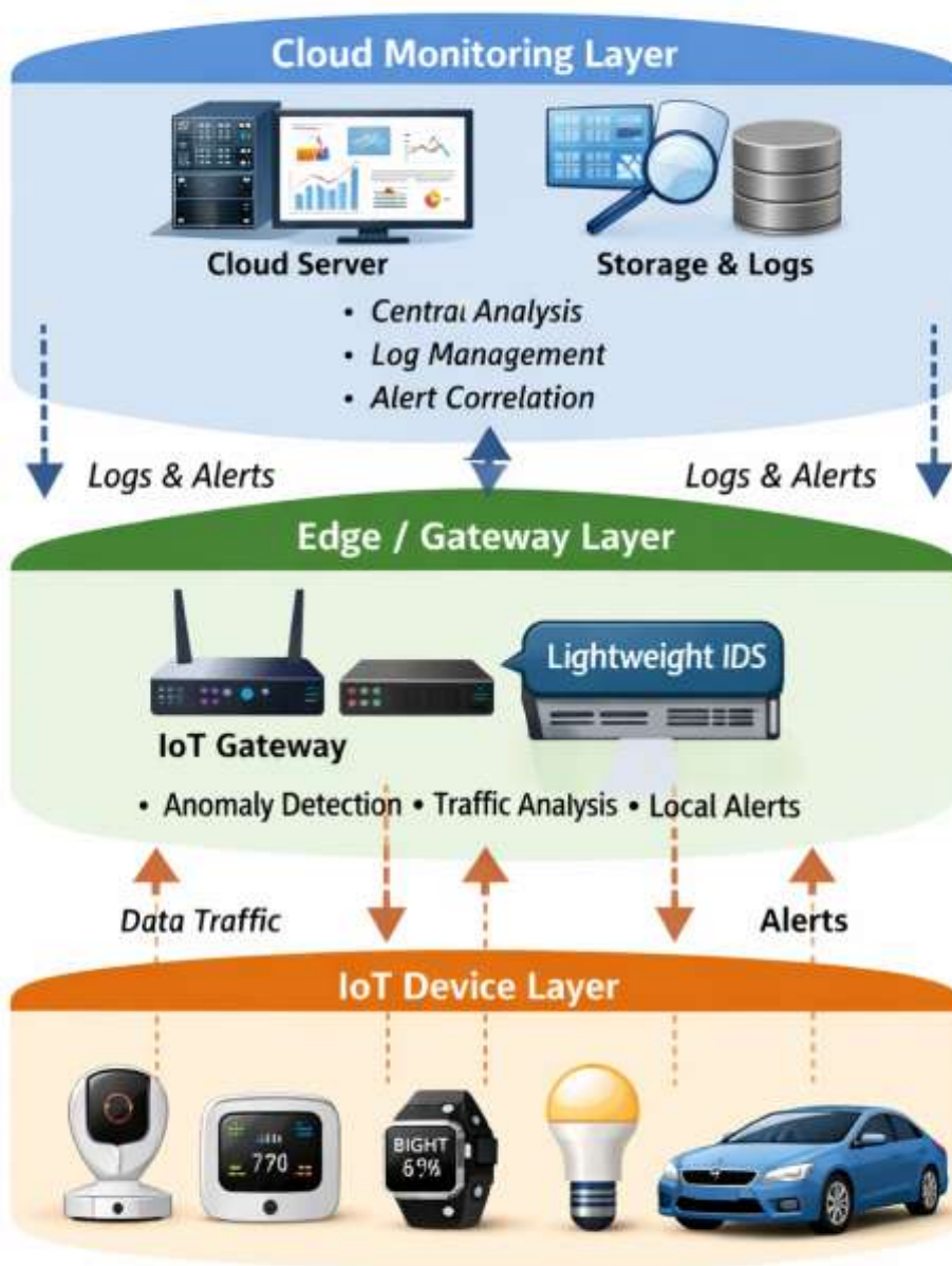
Figure 1: System architecture of the proposed IoT intrusion detection framework.
