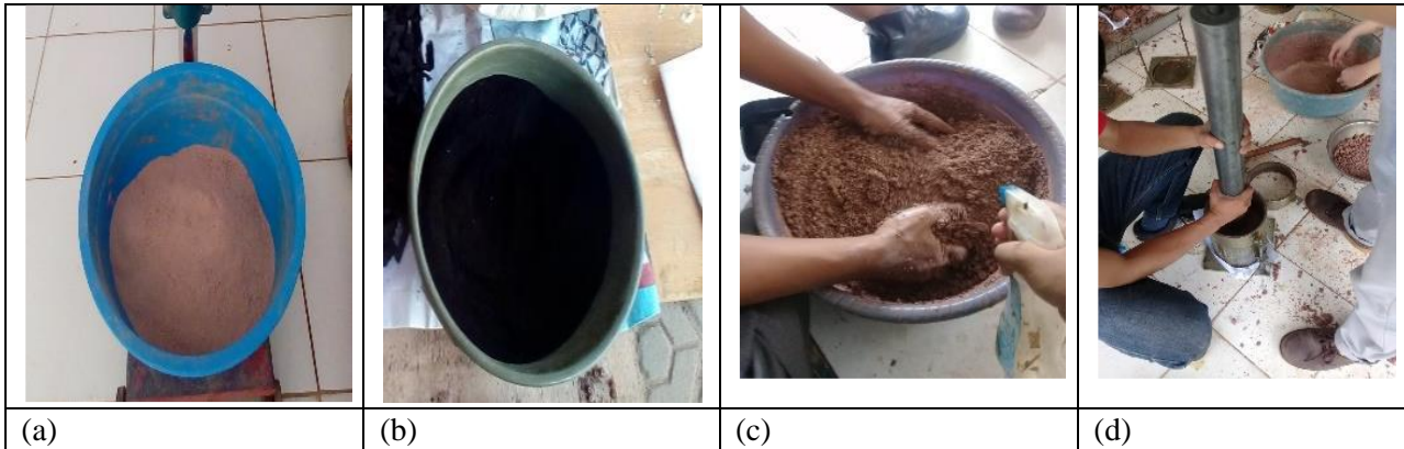
Figure 3. Samples Preparation For CBR Testing (a) Clay (b) Bamboo Charcoal (c) Mixing (d) Compaction
