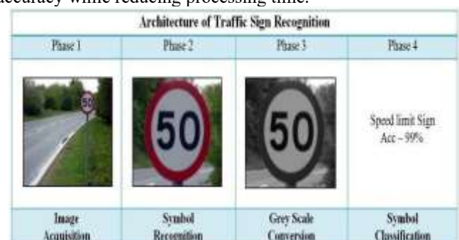
Fig- 3: Architecture of traffic sign recognition system
