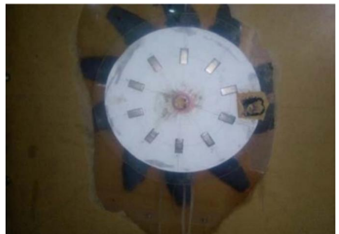
Figure 5. Rotor (N50 Neodymium magnet).
