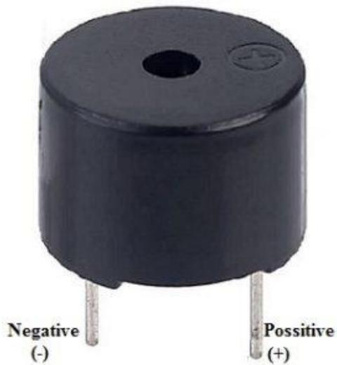
An active buzzer sensor module has a built-in oscillation circuit, thus the sound frequency is fixed. It is able to generate the sound itself. So, you can simply turn it on and off with an Arduino pin, just like the way of turning on and off a Led which is connected to Arduino board.
