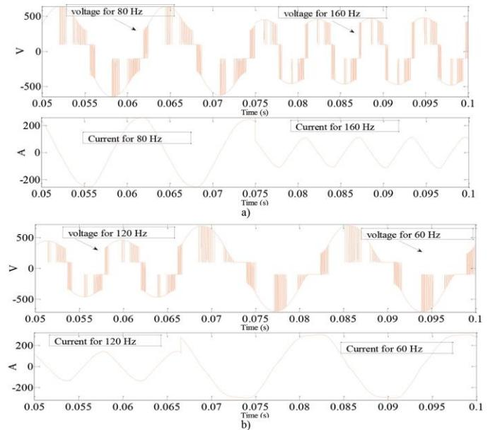
**Fig -13:** The voltage and current on RL load: a) for 80 Hz and 160 Hz b) for 120 and 160 Hz.
