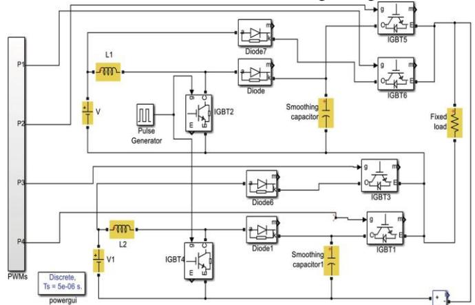
**Fig -4:** Multi-level inverter with reverse connected dual dc-dc converter for simulation.
