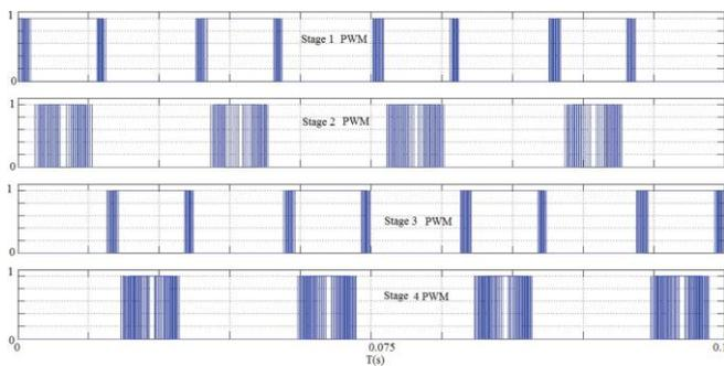
**Fig -2:** Shows the pulse width modulation (PWM) signals controlling the inverter circuit.
