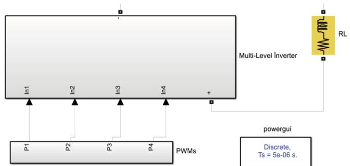
Fig -11: The subsystem created for multilevel inverter in the proposed circuit at the Matlab Simulink.
