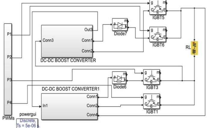
Fig -10: The subsystem created for the converter circuits in the proposed circuit at the Matlab Simulink.
