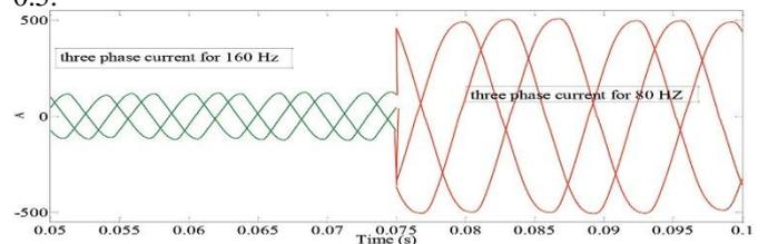
**Fig -19:** The alternating currents for 80 Hz and 160 Hz when the converter units working with the modulation index of 0.8.
