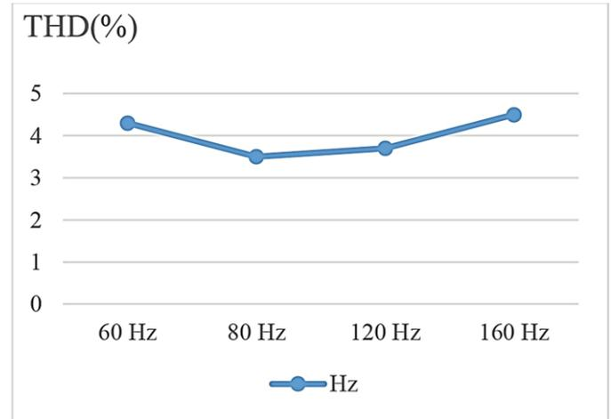
**Fig -17:** Total Harmonic Distortions of the currents formed on the RL load in different frequencies.
