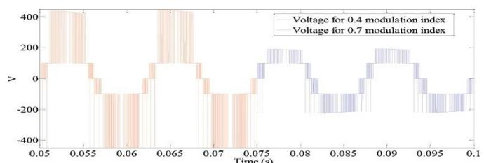
**Fig -6:** Alternating voltage for the 0.4 and 0.7 modulation indexes.
