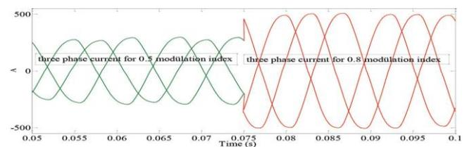
**Fig -18:** The alternating currents at 80 Hz when the converter units working with the modulation index of 0.8 and 0.5.
