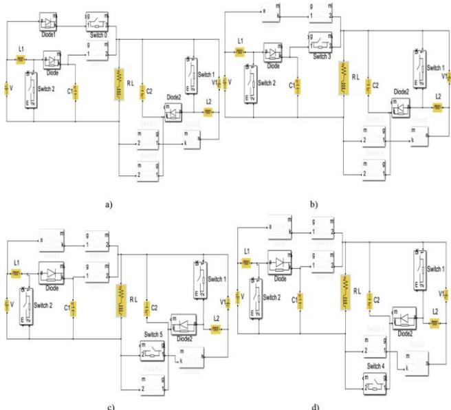
**Fig -3:** Four different circuits for four different times, a) stage 1, b) stage 2, c) stage 3, d) stage 4.
