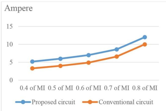
Fig -8: Currents on load for modulation index.
