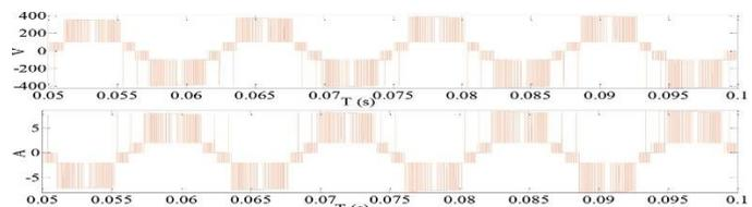
**Fig -5:** The voltage and current for 0.6 of modulation index on the load.
