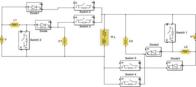
**Fig -1:** The multi-level inverter circuit with the reverse connected double dc-dc converter.
