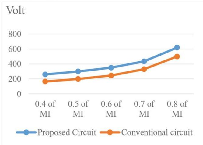
Fig -7: Voltages on load for modulation index.
