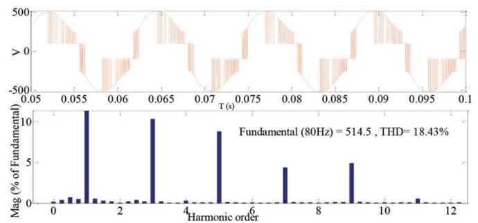
**Fig -14:** Alternating voltage and THD.
