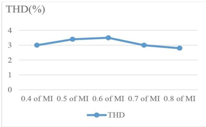
**Fig -16:** Total Harmonic Distortions of the currents formed on the RL load in different modulation indexes.
