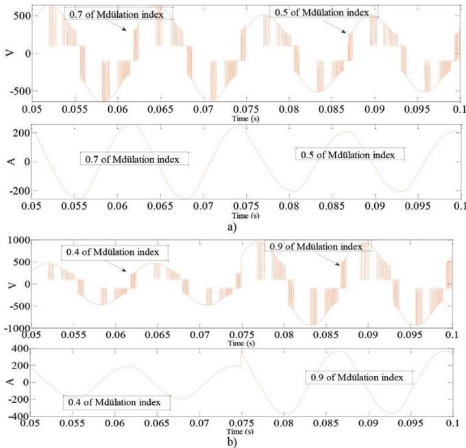
**Fig -12:** The voltage and current on RL load a) for 0.7 and 0.5 modulation indexes b) for 0.7 and 0.5 modulation indexes.
