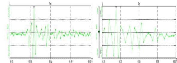
**Acceleration response on the engine head at 750 rpm – Normal rubber (left), composite (right)**
