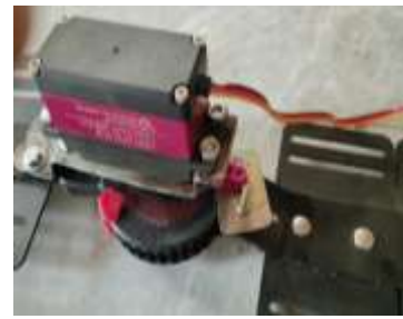
Fig. 1(c) – Servo Motor Mounting on Thigh Frame
