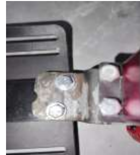
Fig. 1(d) – Servo Horn and Knee Joint Coupling
