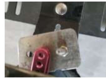
Fig. 1(c) – Servo Motor Mounting on Thigh Frame
