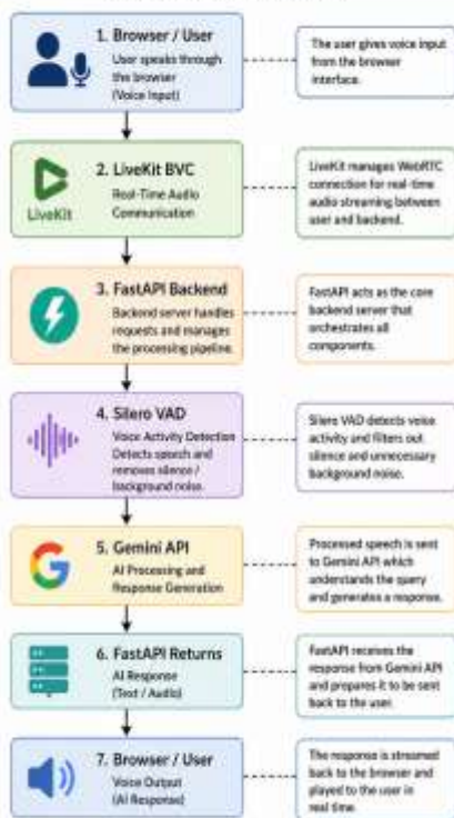
System Architecture of Real-Time Voice Assistant using FastAPI and LiveKit
