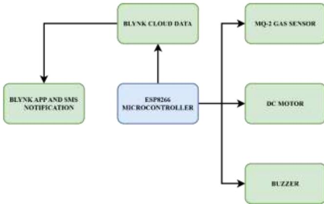
Fig-6: Block Diagram
