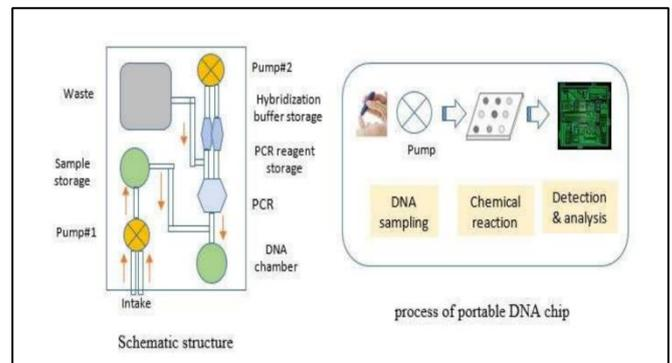
Fig no. 4 Prototype of portable DNA Chip
