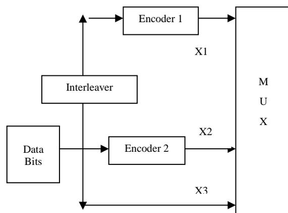
Fig.1 Structure of Turbo Code Encoder [11]
