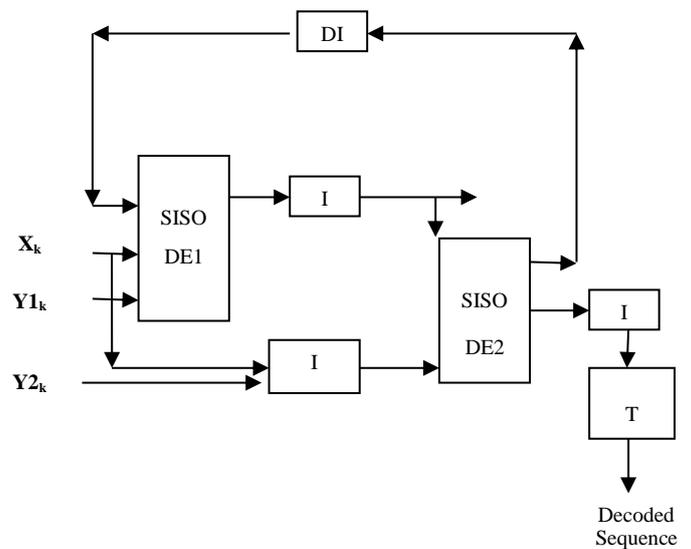
**Fig. Structure of Turbo Decoder [11]**
