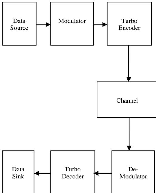
**Fig.2 Use of Turbo Encoder and Decoder in Communication System**
