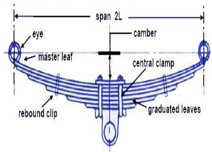
Fig.1 Dimensions of Leaf Spring [1]
