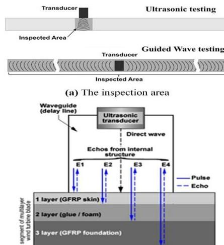
Fig.1 Principle of the pulse echo technique
