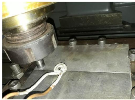
Figure Induction assisted friction stir welding setup [237]
