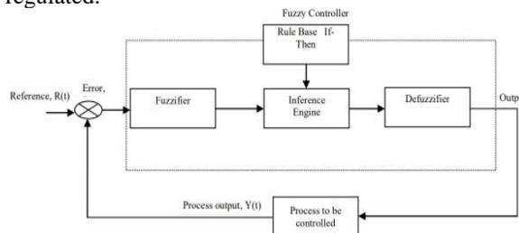
Figure 4. Basic Fuzzy Logic Controller
