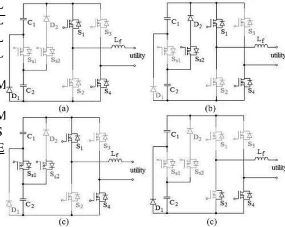
Fig. 7. In the positive half cycle, the seven-level inverter operates in modes 1–4.
