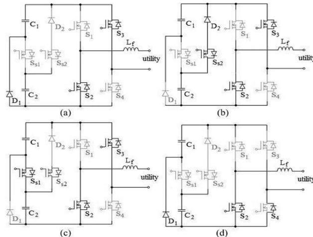
Fig. 8. In the negative half cycle, the seven-level inverter
