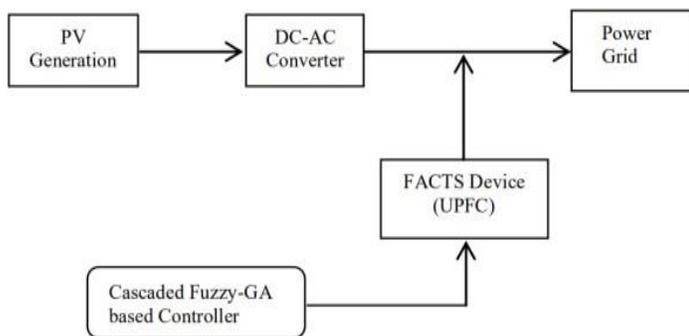
Figure 6. Grid Connected PV system with Proposed Controller and FACTS device
