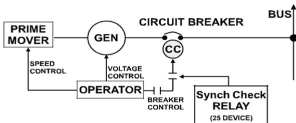
Figure.9 Manual synchronizing with synch check relay
