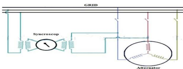
**Figure.6** Synchronization of Alternator Using Synchroscope
