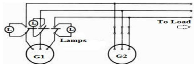
**Figure 4:** Synchronization of generators by 3 dark lamps method
