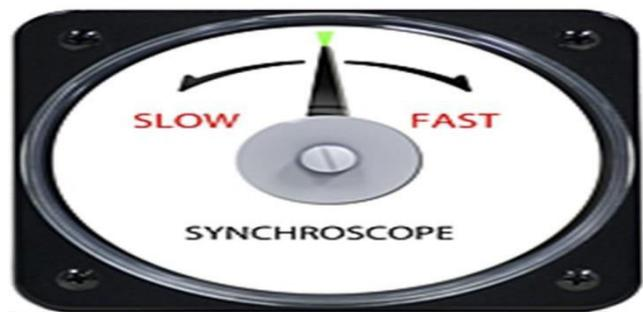
**Figure7** Synchroscope meter and synchronizing indicator
