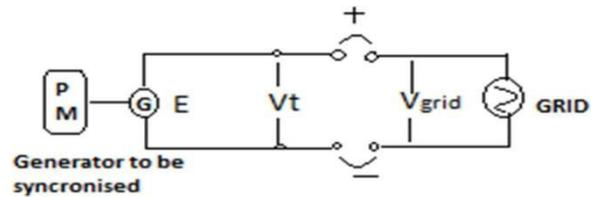
Figure 1 – Generator and Grid Synchronization.
