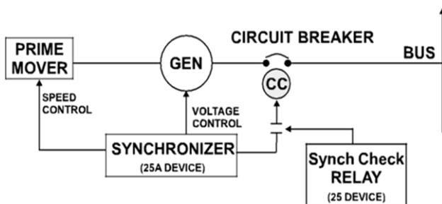
Figure.10 Automatic Synchronizing
