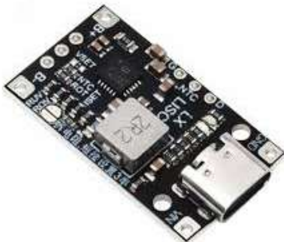
Fig- 5 : BMS Controller
