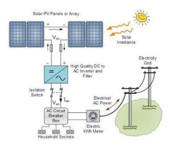
The photovoltaic power plant, primary type of sun powered energy, is an immediate technique for changing over the sun powered radiations into power. Photodiodes are utilized in these plants for the effective assimilation of daylight. This entire framework is for the most part created of battery powered battery, regulator, inverters, load bank and so on PV power plants can be utilized as independent wellspring of energy and it can likewise be associated with primary power lattice.
