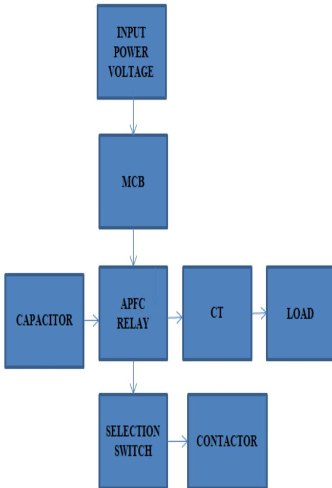
Fig -2: Working System Block Diagram
