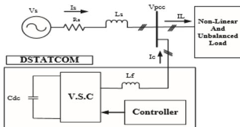
Proposed system introduces a new concept of DTATCOM that Use conventional FACTS and D-FACTS devices. The DPFC gives the possibility of control all system parameters, such as line impedance and power angle, mitigate sag, swell and Harmonics. At the same time, it provides higher reliability and lower cost.
