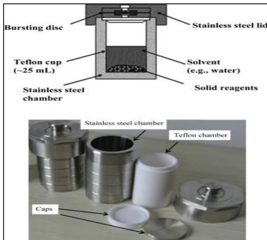
Fig. 2.3 Image of Teflon coated stainless steel autoclave
