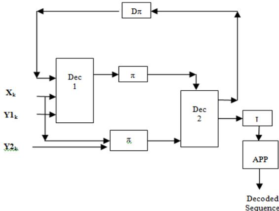
Fig.3 Structure of Turbo Decoder
