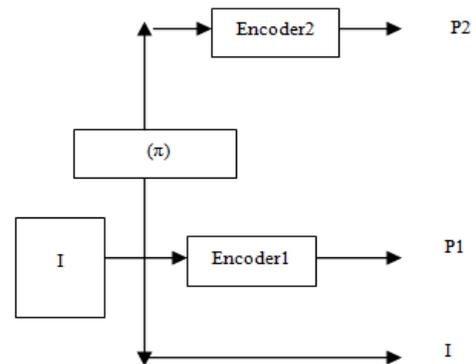
Fig.2 Structure of Turbo Code Encoder
