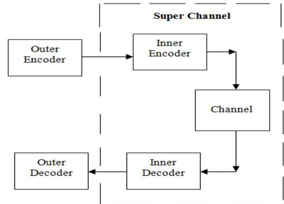
Fig.1 Encoder-Decoder Structure
