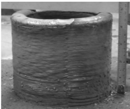
Figure 5: Low carbon steel made from WAAM [2]
