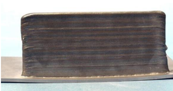
Figure 5: Low carbon steel made from WAAM [2]
