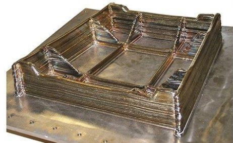
Figure 7: Titanium alloy made from WAAM [3]
