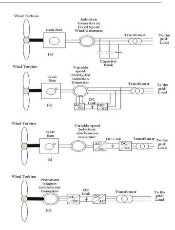
Fig. 8. Power electronics converters in WECS
