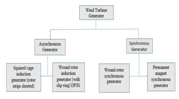
Fig. 7. Various commonly used wind turbine generator
