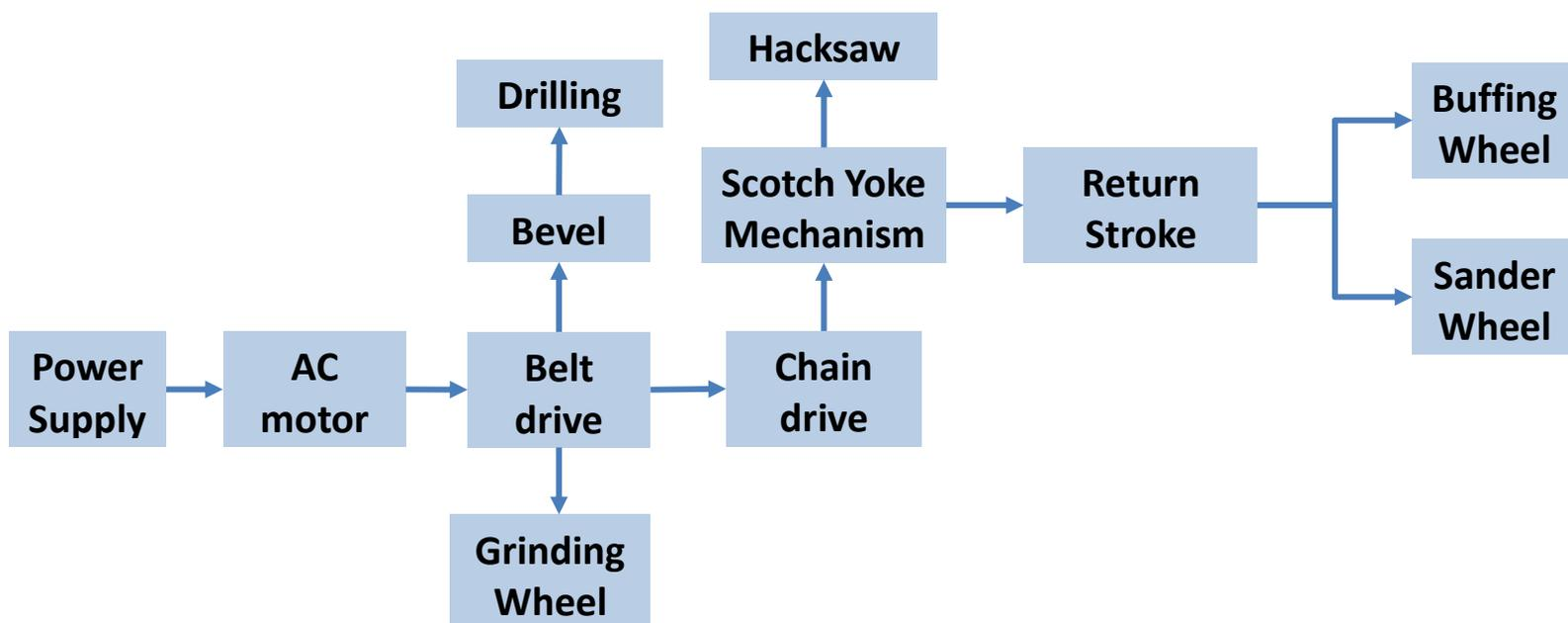
Fig. 15: Working Block Diagram
