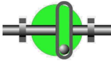
Fig. 03: Scotch Yoke Mechanism
