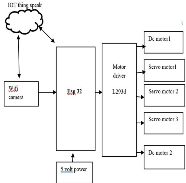
Figure1: Block Diagram of IOT Based Snake Robot.
