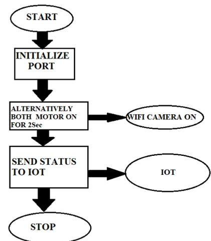
Figure2: Flow Chart of IOT Based Snake Robot
