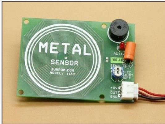
**Fig 7:** Metal detection Sensor
