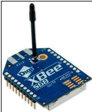
**Fig 10: ZigBee Module**
