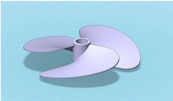
longitudinal axis, giving the propeller an overall cup-shaped appearance. This design preserves thrust efficiency while reducing cavitation's, and thus makes for a quiet, stealthy design.
