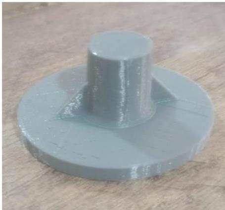
**Figure 8** Tibial component
