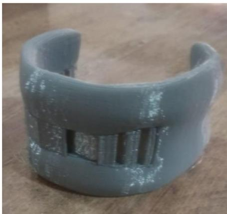
Figure 6 Femoral component
