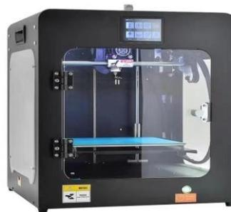
Figure 5 FDM 3D Printing Machine
