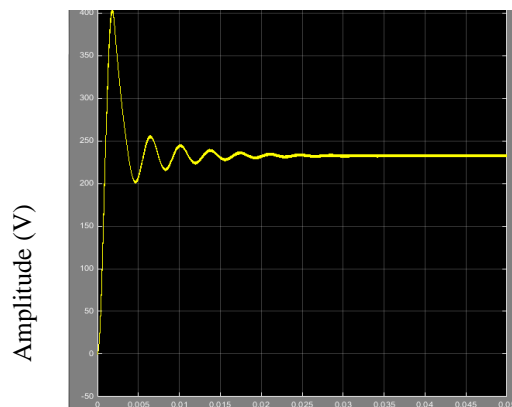
Figure 5. (b) Simulated response of Buck Boost converter in Boost Mode
